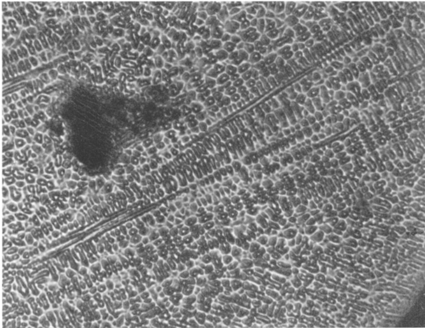
Figure 2 Photomicrograph of an undercooled particle of VM300 maraging steel atomized in argon ( \times 250 ).
